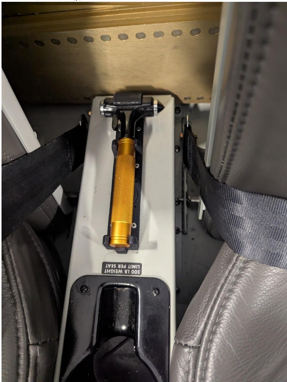
FIGURE 7-14 EXAMPLE EGRESS HAMMER LOCATION
