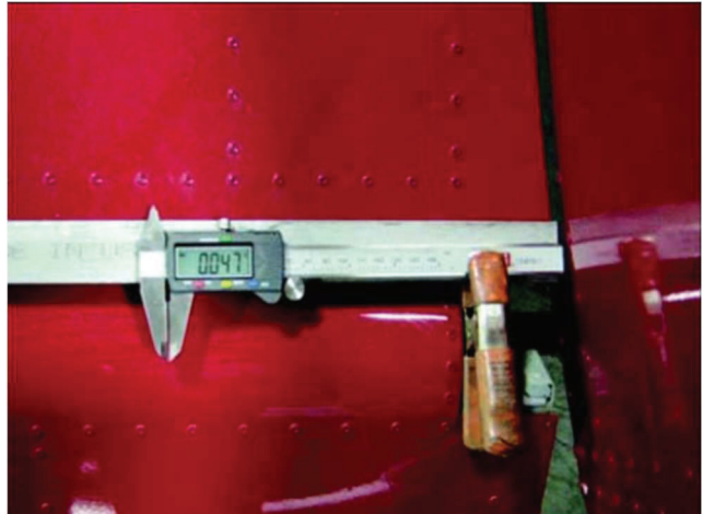
Figure 7.1: Inspect Rear Spar Doubler
