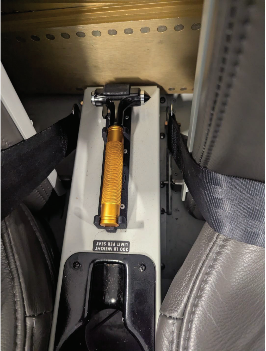
FIGURE 7-13 EXAMPLE EGRESS HAMMER LOCATION
