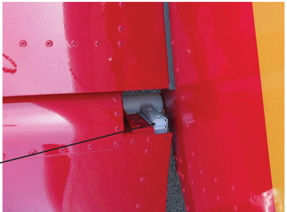
FLAPERON TAB FULLY ENGAGED IN ACTUATOR SLOT
