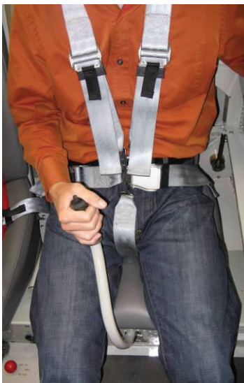
Left Flaperon: DOWN Right Flaperon: UP Stabilator: UP
