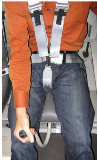
Left Flaperon: DOWN Right Flaperon: UP Stabilator: DOWN
