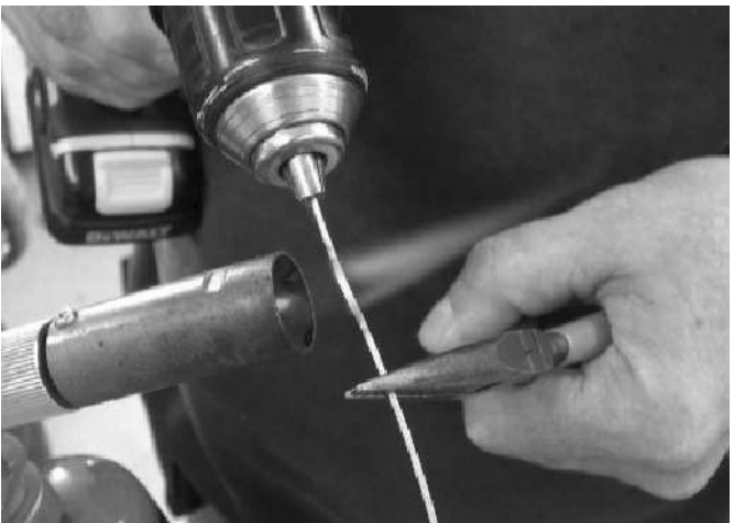
FIGURE 3: TWIST-WELDING PUSH-PULL CABLES
