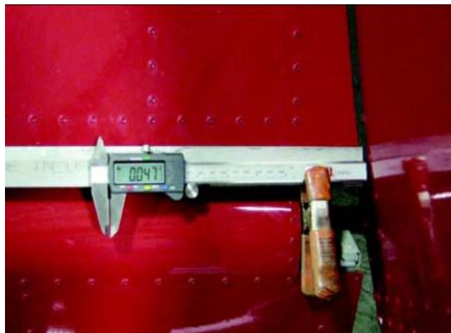
Figure 7.1: Inspect Rear Spar Doubler
