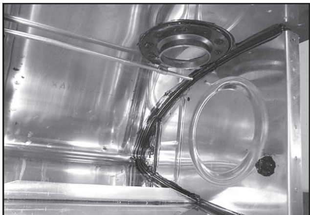
Fig. 7-8. The interior of the tank at the outboard end. The T-410 reinforcement helps seal around the nose. The blob on the rib is a 316" rivet set in the tooling hole and covered with sealant. The filler neck and vent line are also visible.
