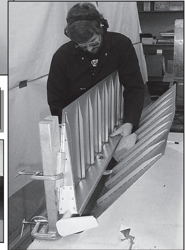
Above: Using a piece of aluminum angle to hold the trailing edge of the rudder straight during bonding and riveting. One straight piece, the full length of the rudder, is required...the short piece is just for the photo.
