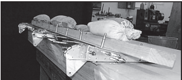
Fig. 7-23. The top skin is held down with a board and weights.
