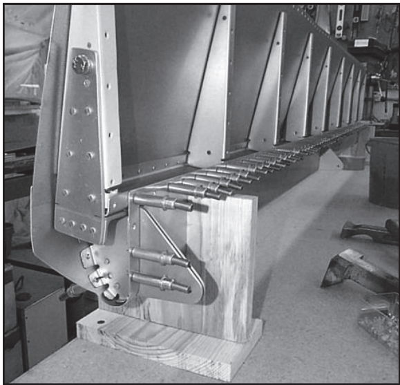
Fig. 7-27. The flap assembly is inserted into the "saddle" fixture for riveting.
