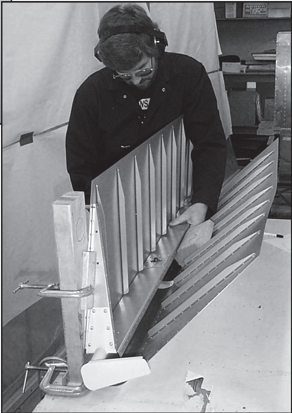
Above: Using a piece of aluminum angle to hold the trailing edge of the rudder straight during bonding and riveting. One straight piece, the full length of the rudder, is required...the short piece is just for the photo.
