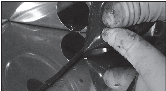
Fig 7-10. A bead of sealant for the rear baffle is squeezed out of a plastic bag.
