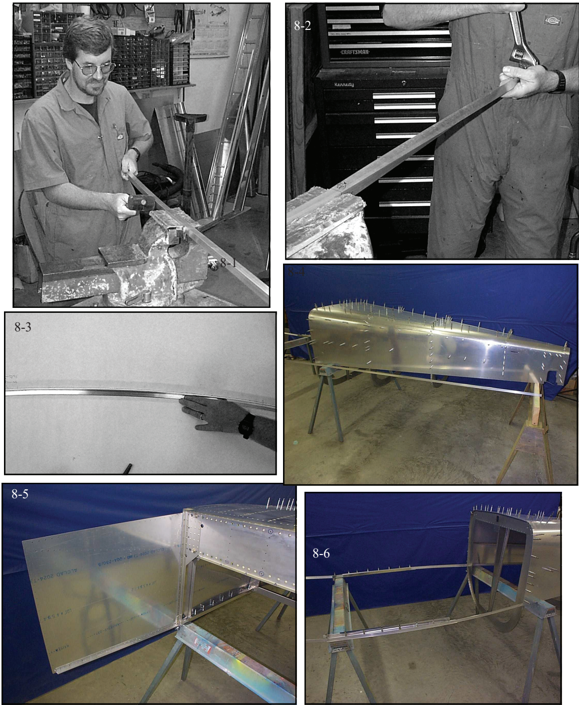
Fig 8-1. Bending the longeron in a vise. Fig 8-2. Twisting the longeron. Fig 8-3. Checking the longeron against the template. Fig 8-4. The aft fuselage bulkheads and skins riveted together. Fig 8-5. The forward side skin attached to the forward fuselage. Fig 8-6. The longerons inserted. Fig 8-7. Interior of the tailcone with floor ribs clecoed in place.
