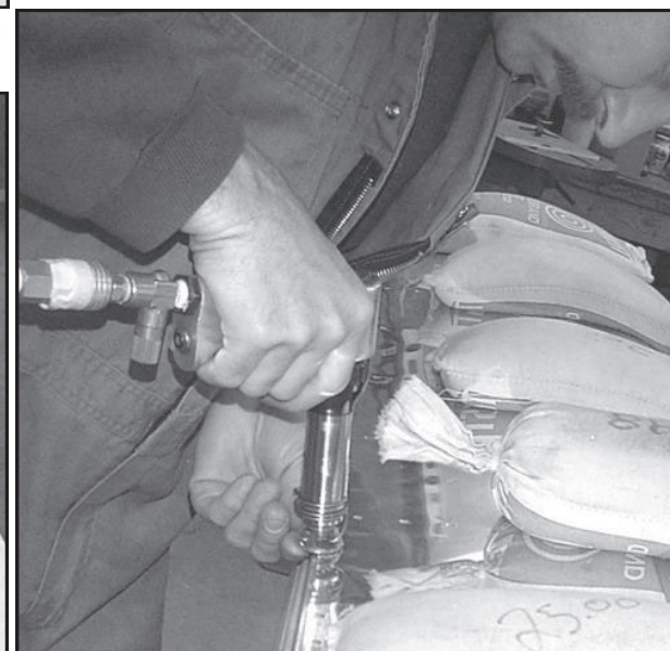
Fig. 7-19. Finishing the trailing edge rivets, using a mushroom set and a back-riveting plate set into the table.
