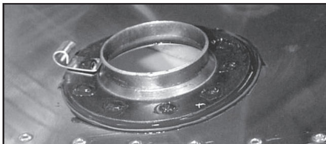
Fig 7-9. The filler neck riveted to the inside of the tank skin. A common rivet holds the T-914 clip to secure the vent line.
