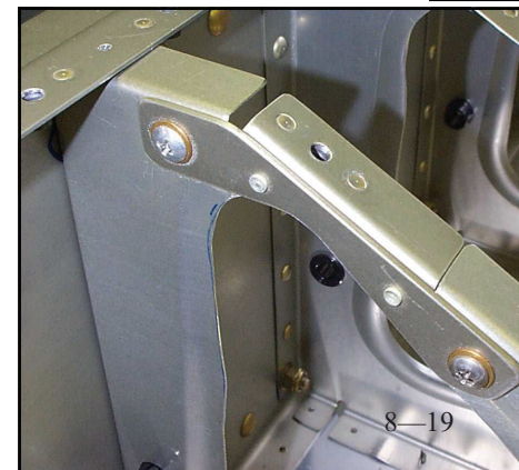
Fig 8-14. The F-656 gusset. Fig 8-15. The F-634 seat belt anchor. Fig 8-16. The F-838B cover support rib. Fig 8-17/18. Details of the F-729/730/705 junction. Fig 8-19. The modified F-916 floor rib
