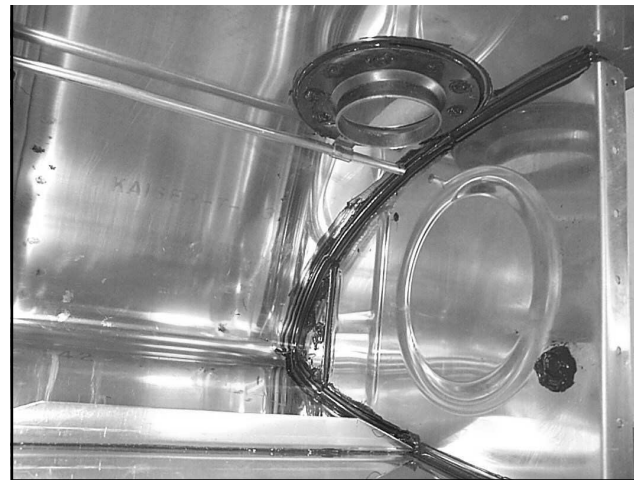
Fig. 7-8. The interior of the tank at the outboard end. The T-410 reinforcement helps seal around the nose. The blob on the rib is a 316" rivet set in the tooling hole and covered with sealant. The filler neck and vent line are also visible.
