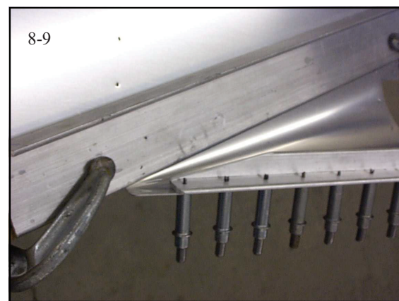
Figs 8-8-11: Various stages of the conical bend on the F-970 side skin. The forward end is bent almost to a sharp corner, but be cautious...if you try to do too much it will crack.
