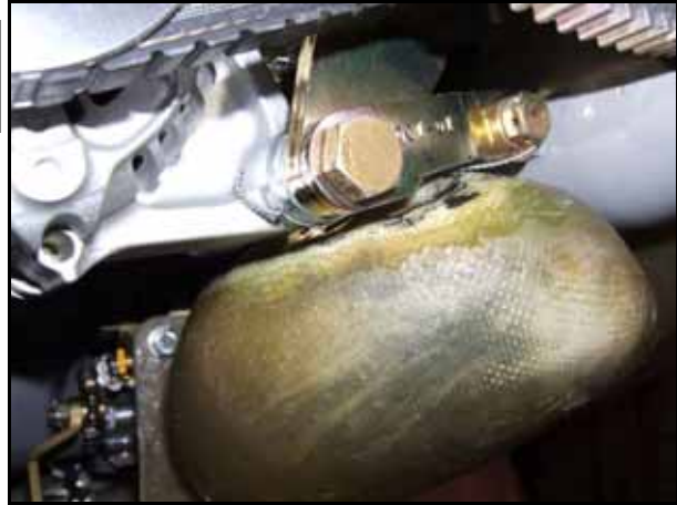
A small depression in the fiberglass "snorkel" provides clearance for the alternator bracket.
