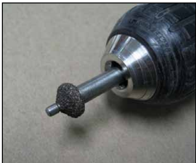
Permagrait countersinking tools won't fit in a microstop cage, but you can countersink fiberglass by eye accurately enough.
