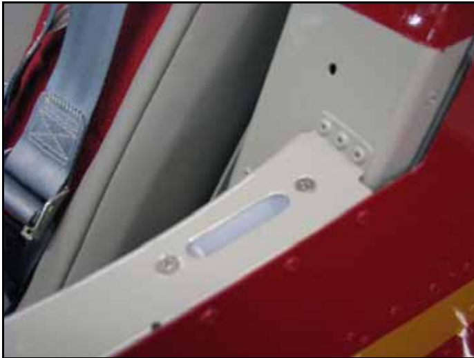
Top left: Behind the seats are the overlapping wing spars — one of the big pins is visible just below the orange ELT — and the fuel tank. Top right: Toe brakes and rudder pedals. Bottom left: The recess in the top canopy deck accepts the tongue of the canopy frame, shown bottom right.
