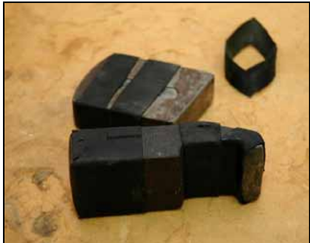
Simple part protectors made from old bicycle inner tubes slip onto almost any bucking bar.
