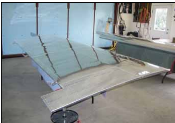
Below: Voila! One hundred and two hours later, the wing panels are done. Construction started April 9 and the wings, except for the flaperons, were ready to fly on April 29. So, five hours a day for three weeks and wings are yours.
