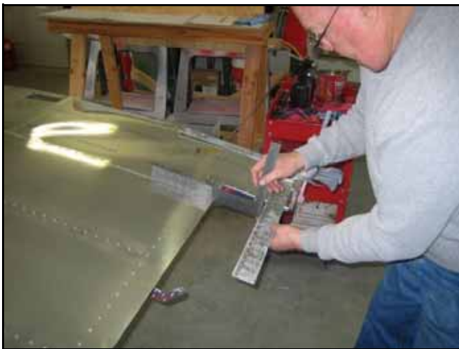
Top: Jim suggests we add an awl to the tool list. He uses it to make fine adjustments to full-size pre-punched holes.
