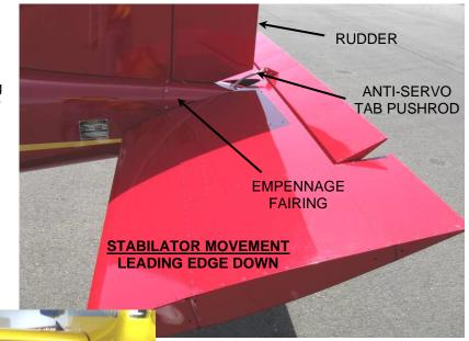
Anti-Servo Tab – CHECK condition, proper attachment
