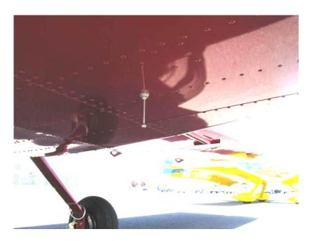
• Muffler – CHECK condition, security of attachment
