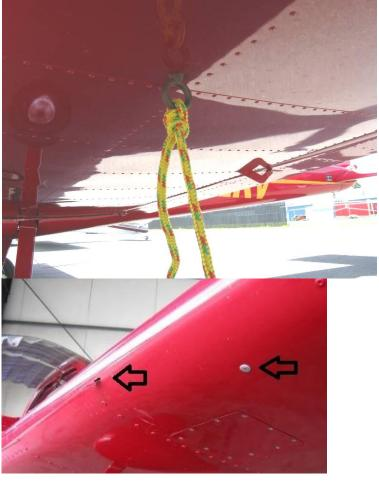
Wing Hand Hold - APPLY FORCE fore/aft & up/down; CHECK no free movement.
