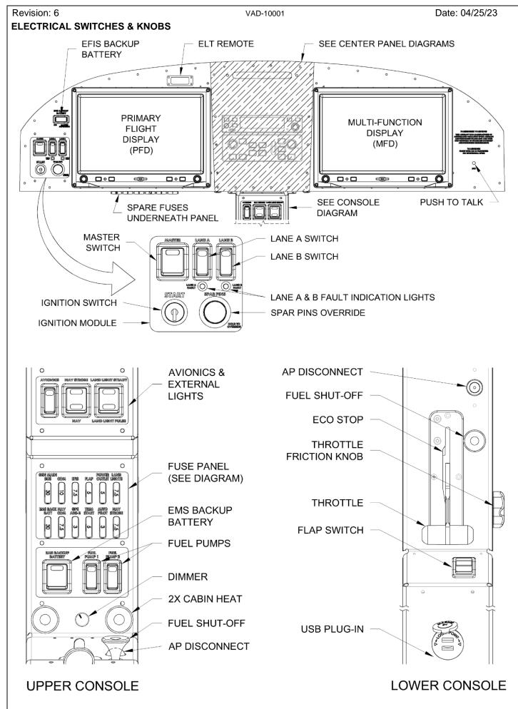
SWITCH LIGHTING: Except for the keyed starter switch and the Garmin EFIS backup battery switch, all switches are internally lit. If the optional lighting kit is installed, turning on the NAV lights will also light a LED eyeball light located on the roll bar that is used to illuminate the panel area (including the unlighted switches) during night flight.
