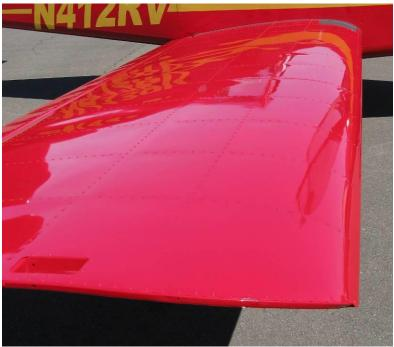
Wing Hand Hold – APPLY FORCE fore/aft & up/down; CHECK no free movement.
