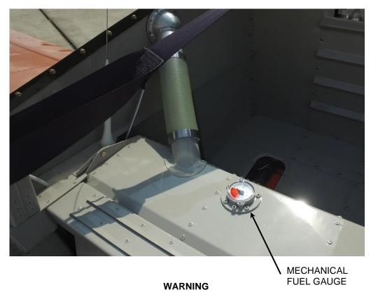
Sample the fuel to remove contaminates (mainly water) <u>before</u> the fuel pumps are turned on. The high flow rate of the fuel pump(s) (especially for the 912 iS) will emulsify the water into the fuel making removal impossible.
