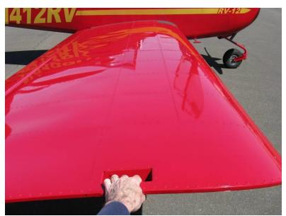
Tie-Down – UNTIE the tie-down rope/chain, REMOVE eye bolt if desired. Ensure eye bolt is secured in the wing if not removed.
