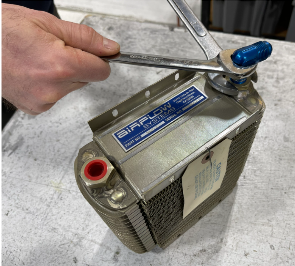
FIGURE 1: USE TWO WRENCHES WHEN TIGHTENING FITTINGS
