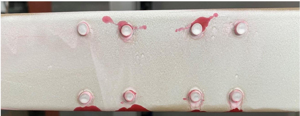
FIGURE 4: EXAMPLE 2 - CRACK LOCATIONS - FWD SIDE OF SPAR
