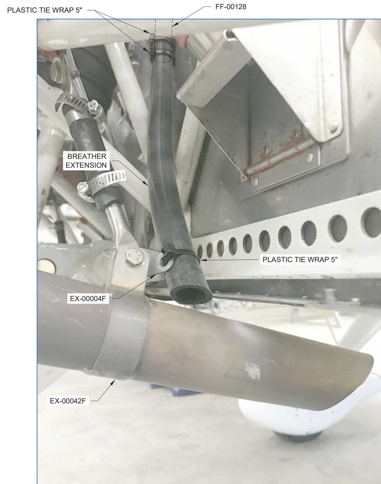
FIGURE 1A: BREATHER EXTENSION ROUTING
