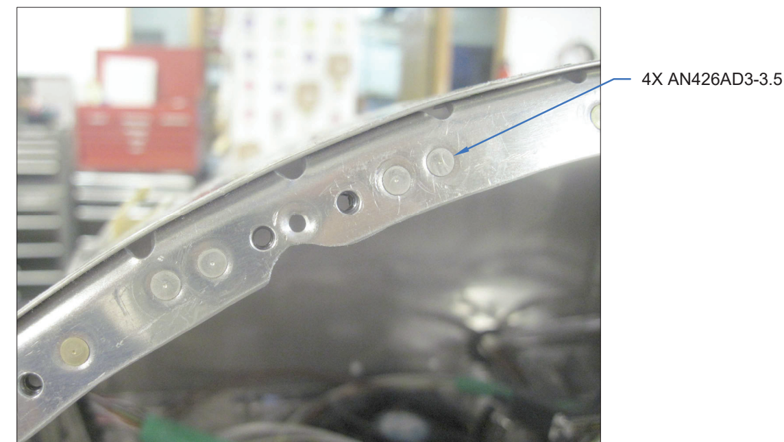
FIGURE 3: RIVETING THE NEW NUTPLATES
