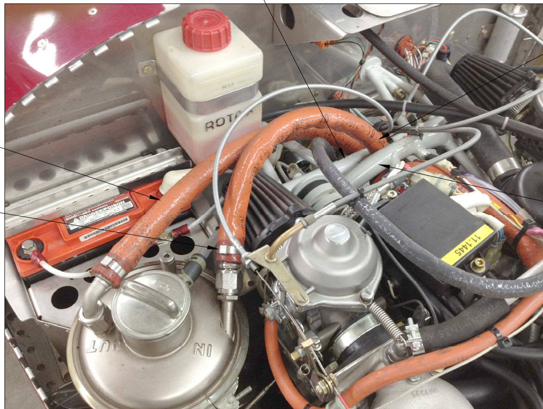
FIGURE 2: INSTALLING THE OIL HOSES VIEW FROM ABOVE
