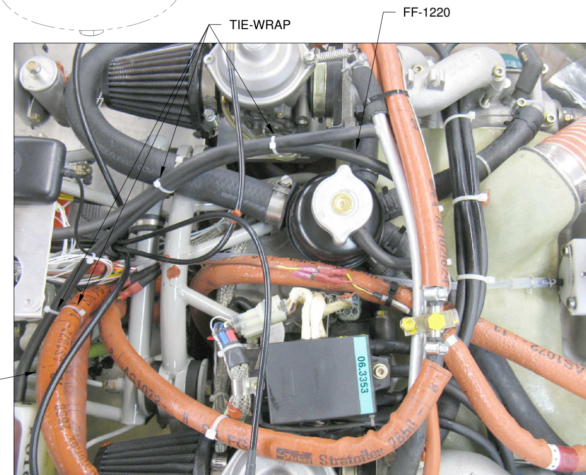
FIGURE 2: OVERFLOW BOTTLE HOSE ROUTING
