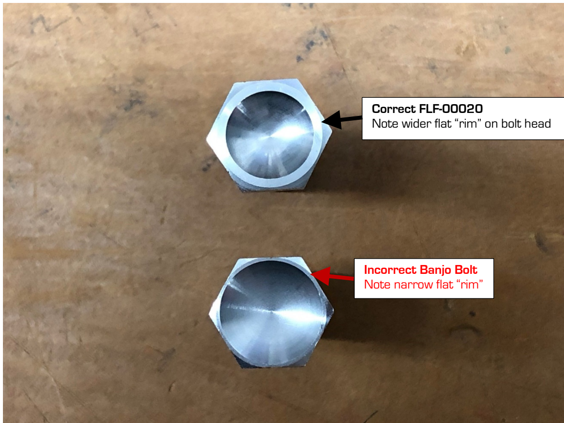
Figure 1: Banjo Bolt Head Details
