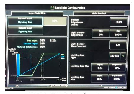
FIGURE 4: G3X Backlight Configuration
