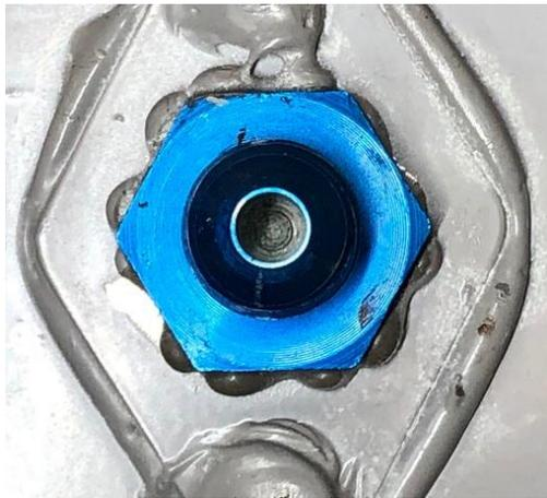
**FIGURE 2:** AN832-4D bulkhead fitting with blocked opening
