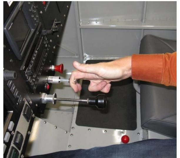
Fuel shut-off valve is used to permit or prevent fuel from flowing to the engine compartment. It may be pulled up to the 'OFF' position to prevent fuel flow, or pushed down to the 'ON' position.
