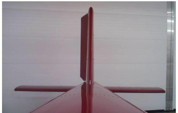
Rudder pedals and related Rudder movement
