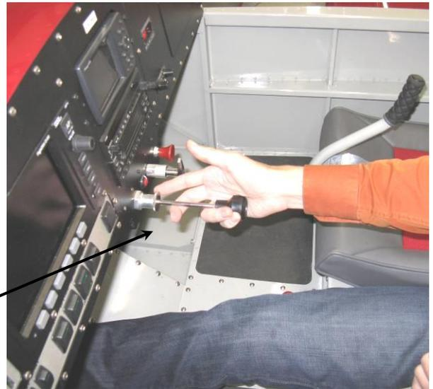
Choke is used for cold starting. The choke can be locked in a specific position by rotating the 'T' handle.
