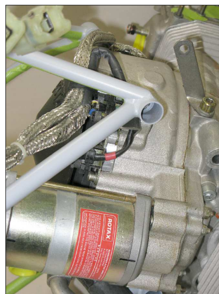
FIGURE 3: INSTALL ENGINE MOUNT: PART 1
