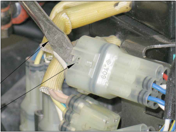
FIGURE 4: SEPARATING CONNECTOR HALVES
