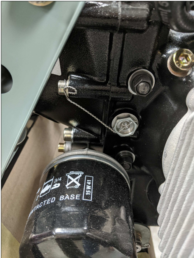
FIGURE 2: SAFETY WIRE MAGNETIC PLUG (912iS SHOWN, SIMILAR FOR 912ULS)
