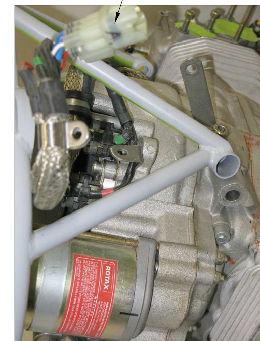
FIGURE 5: INSTALL ENGINE MOUNT: PART 3
