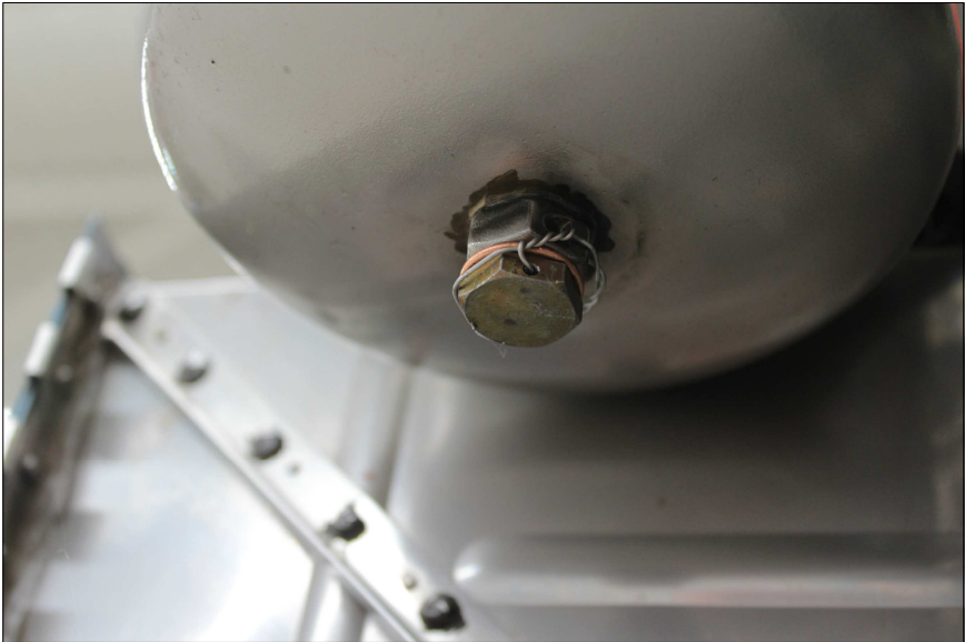
FIGURE 5: SAFETY WIRE OIL TANK DRAIN PLUG
