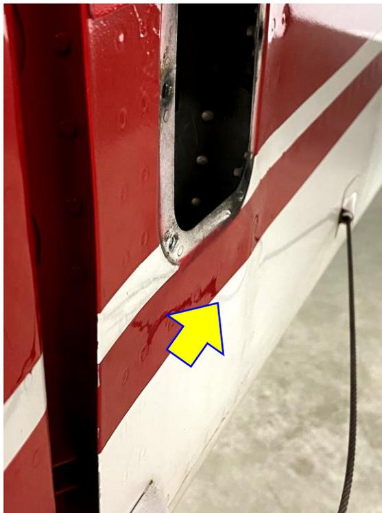
**FIGURE 1:** RV-7 with deformed tailcone skin near access panel.
