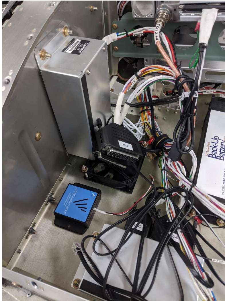
FIGURE 1: SUGGESTED AITHRE MODULE MOUNTING LOCATION (EX 2.0 and Garmin shown, similar for EX 3.0 and/or Dynon)
