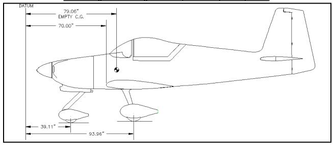
Main wheel, right 93.96" aft of datum. Main wheel, left 93.96" aft of datum. Nose Wheel 39.11" aft of datum
