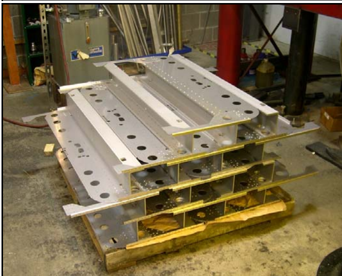
Top: a massive yoke on the pneumatic floor riveter reaches all the driven rivets on an RV-12 center section.
