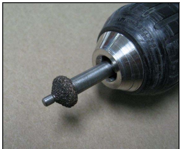
Permagrit countersinking tools won't fit in a microstop cage, but you can countersink fiberglass by eye accurately enough.
