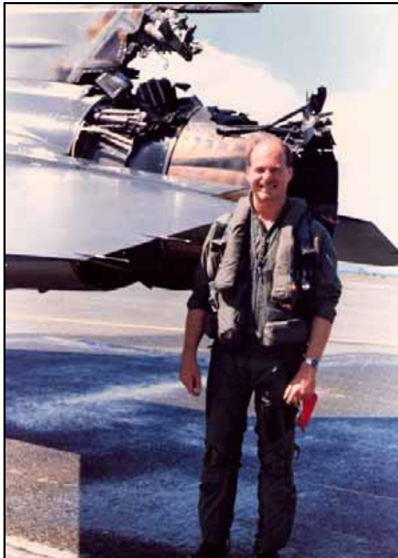
Now you know why they call him Smokey...his airplane caught fire! In this case the board concluded: "The failure of a magnesium alloy restraining band surrounding the afterburner section of the GE F110 engine in Capt Ray's F-16C contributed to the failure and subsequent in-flight fire and ensuing forced flameout landing".
