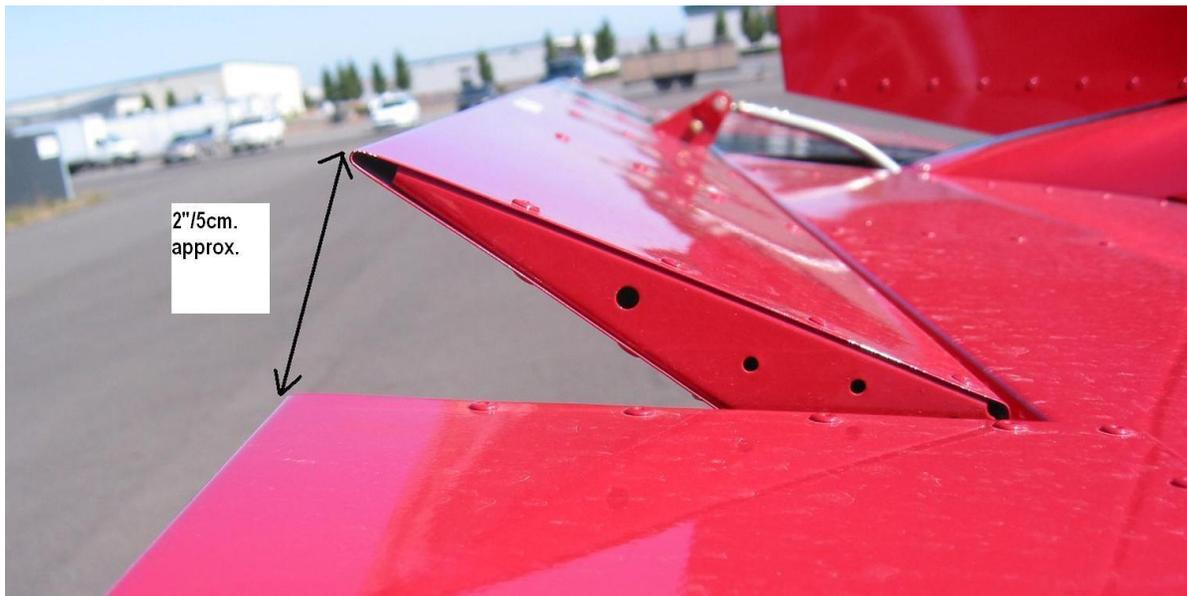
**CAUTION:** The exact neutral trim position for take-off will depend on loading and the individual aircraft. The pilot should be ready to apply forward or aft control pressure as necessary to establish and hold the desired take off attitude.
