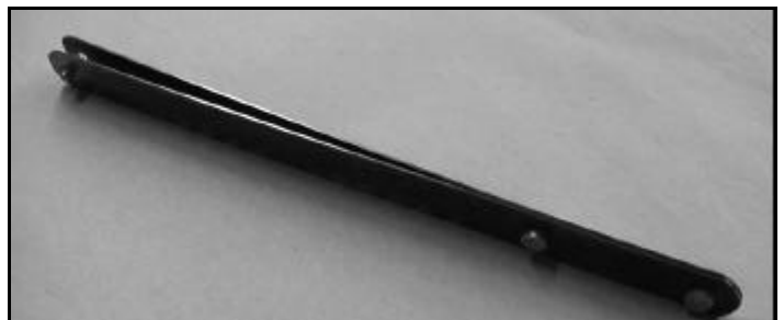
A thin hacksaw blade makes a thin hole-finder, particularly useful for sliding under canopy skirts and locating holes already drilled in the canopy. Find a straight, thin blade, grind the teeth off it, and cut it in half. Align and clamp the halves together and drill two #30 holes near one end, through both halves. Rivet the two halves together. Drill the other end with a single #30 hole. Countersink the inside surface of one strip slightly and insert a AN1097AD4-4 rivet. Set it just enough to make it stay, then file the shank of the rivet until it just fits a #30 hole.
