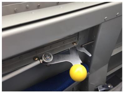
FIGURE 1: CANOPY LATCH PRE ENGAGEMENT OF CANOPY SWITCH
