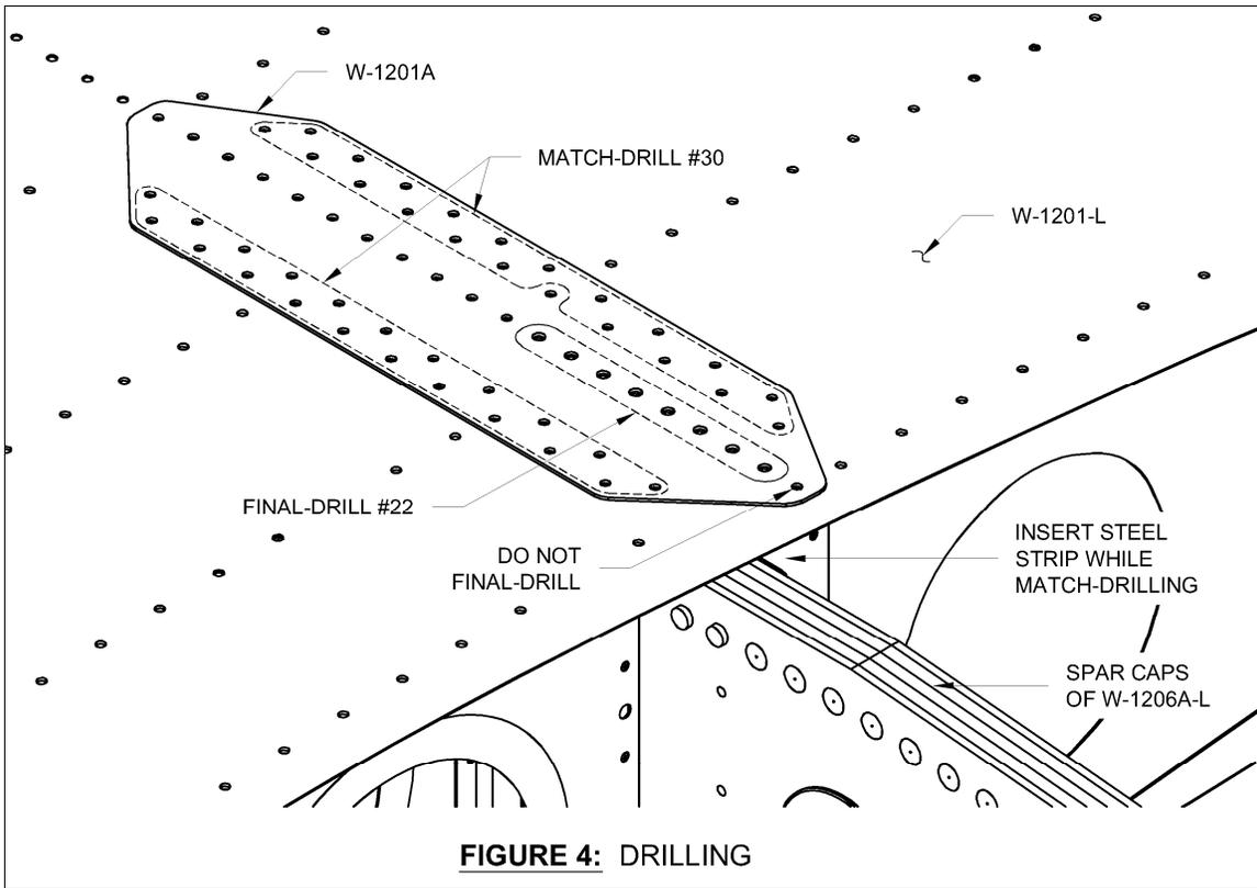
**Step 9:** Remove the doubler and deburr the holes. Confirm that there are no chips trapped between the skin and the spar flange. Any chips or large burrs around the holes that overly the spar caps of the left wing can be knocked off using a chip chaser or the end of a steel ruler.
