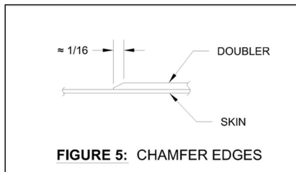
**Step 11:** If desired, prime both sides of the doubler. If a paint coat is desired over the primer, only apply paint to the non-mating surface (the side that will show).
