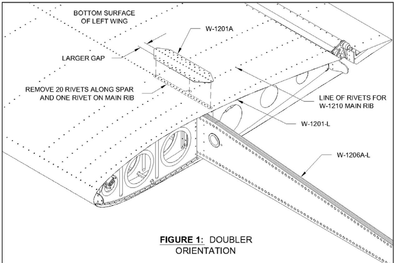
**Step 4:** Depending on the presence and thickness of paint, the rivet heads may stay in place after drilling. Use a 1/8" diam. pin punch to pop the rivet heads off of the skin surface.
