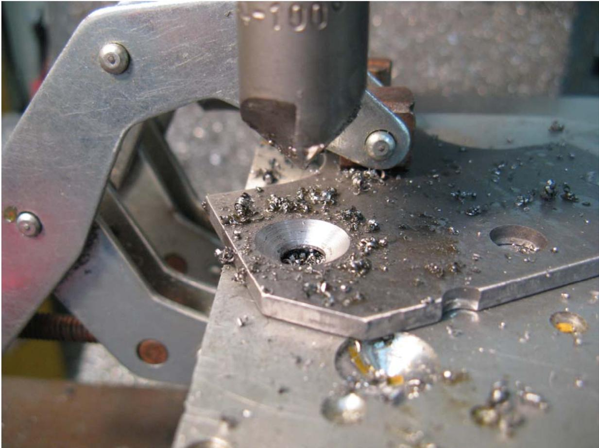
**FIGURE 19:** MACHINE-COUNTERSINKING
