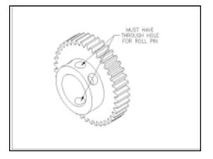
Please inspect your C-1014 spur gears to assure they have been drilled to accept the MS16562-42 roll-pin. If you find that the gears you received are **not** drilled, please return them to Van's Aircraft for replacement.
