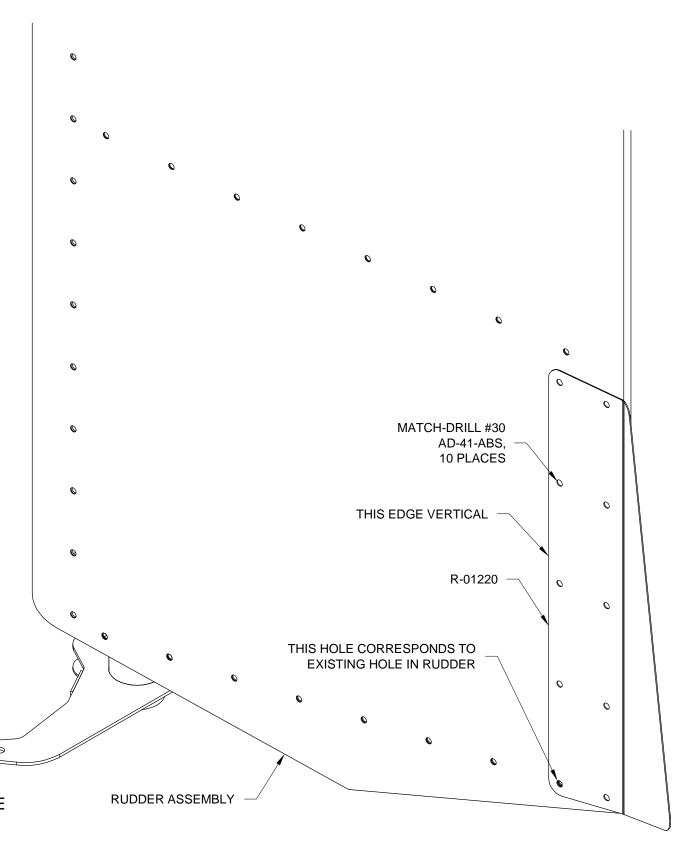
FIGURE 1: INSTALLING THE **TRIM TAB**
