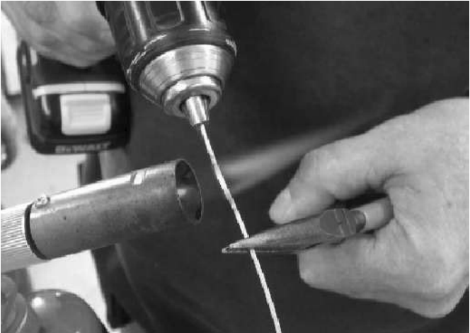
FIGURE 3: TWIST-WELDING PUSH-PULL CABLES Image and process by Brian Carpenter
