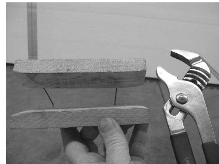
FIGURE 4: TRAILING EDGE TOOL
