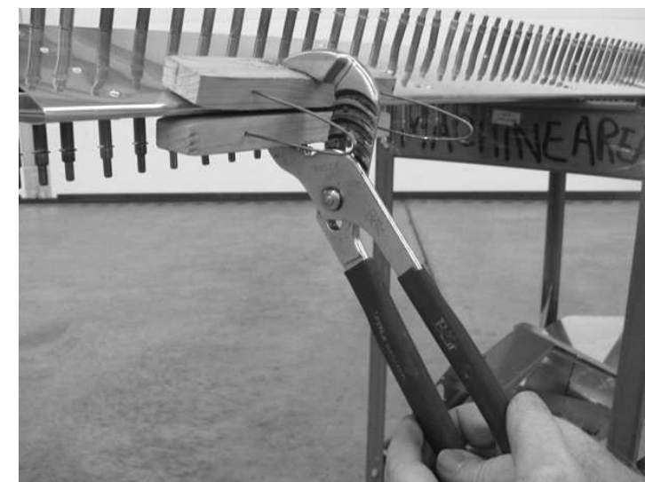
FIGURE 5: TRAILING EDGE TOOL APPLICATION
