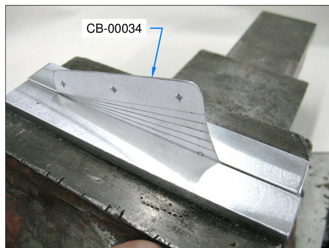
FIGURE 1: BEND LINES 1 TO 6
