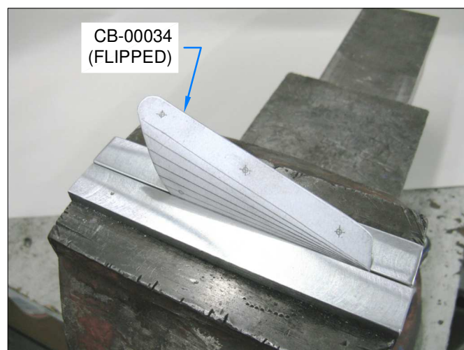
FIGURE 2: BEND LINES 7 TO 10
