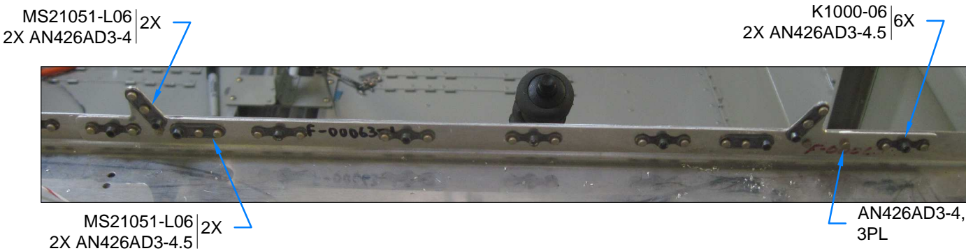
FIGURE 3: INSTALLING THE DOUBLER (VIEW FROM FIREWALL SIDE)
