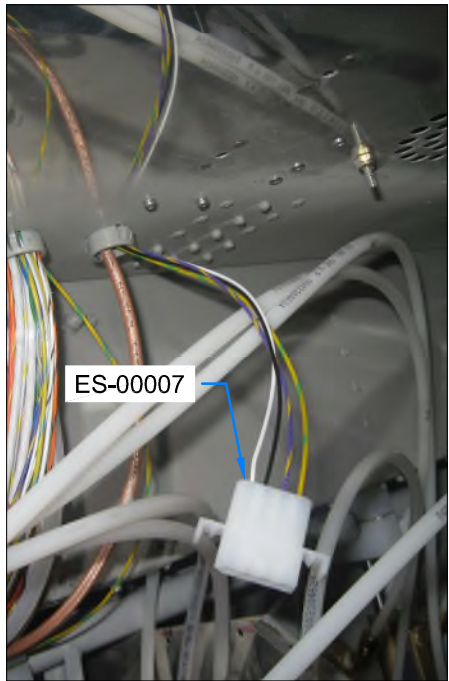
FIGURE 2: ROUTING AUTOPILOT DISCONNECT WIRES
