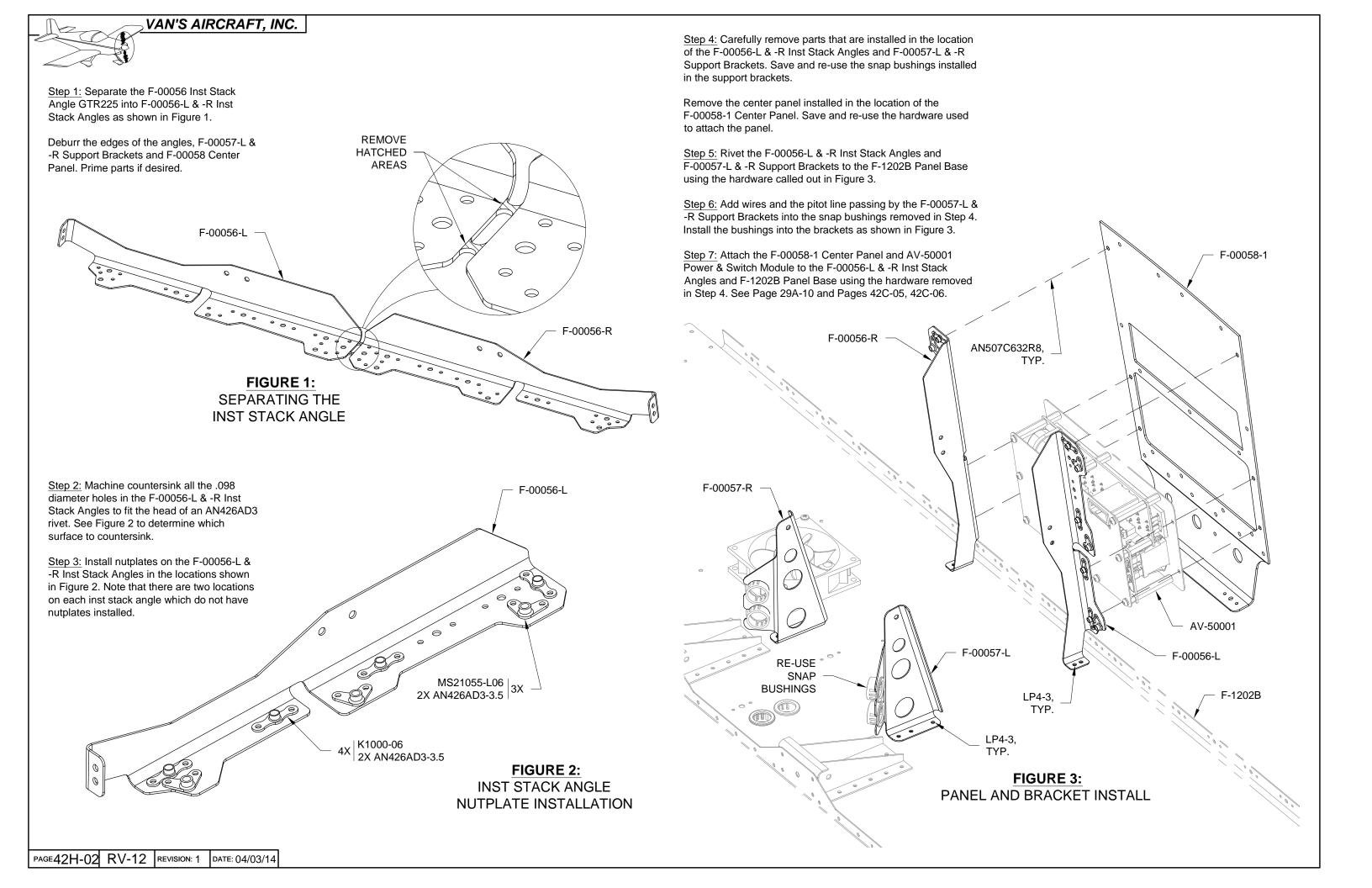
Step 1: Attach the AV GARMIN GTR225 Tray to the F-00056-L & -R Inst Stack Angles and F-00057-L & -R Support Brackets using the hardware called out in Figure 1.
