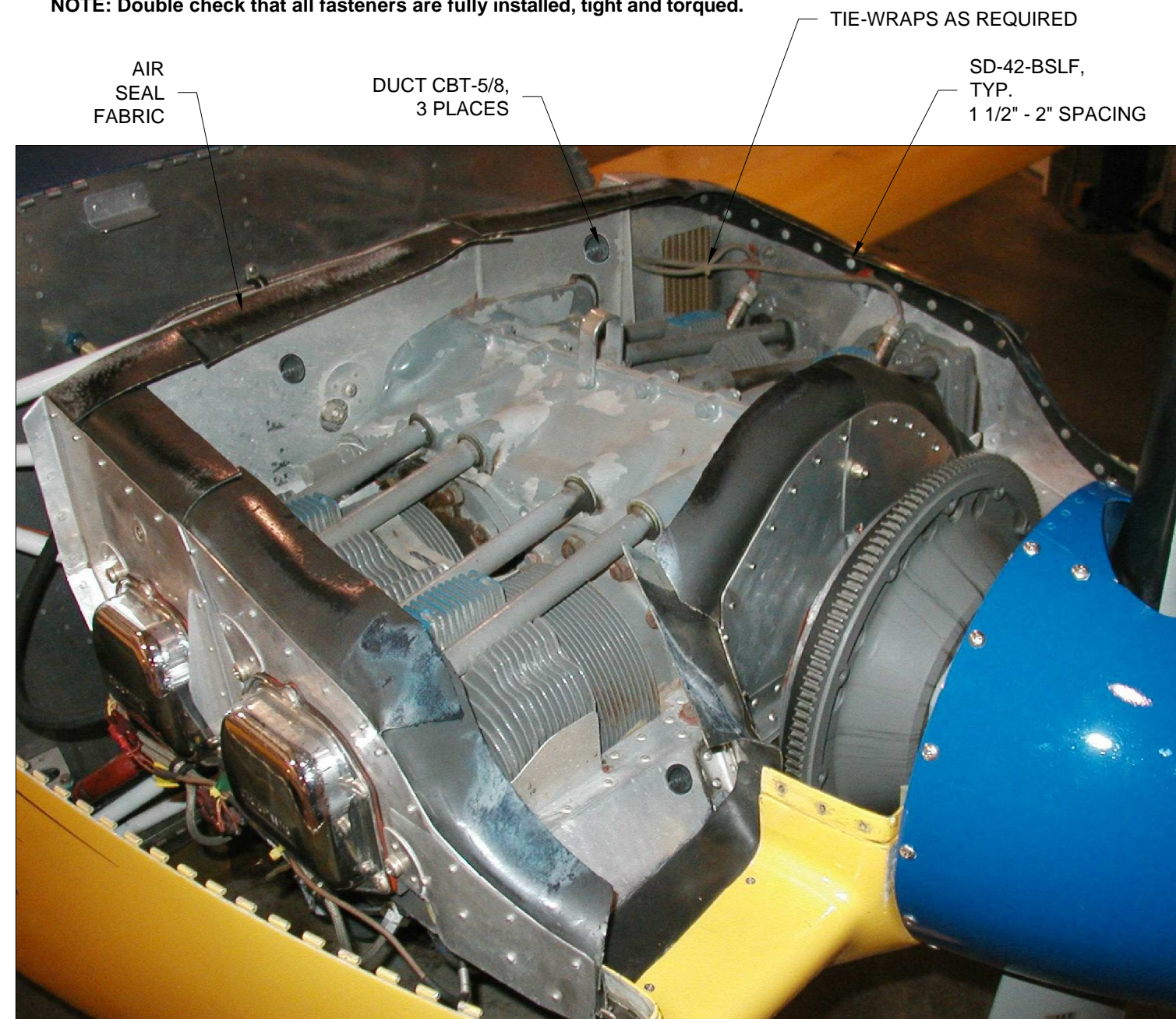
FIGURE 2: AIR SEAL FABRIC - RV-7 VIEW
