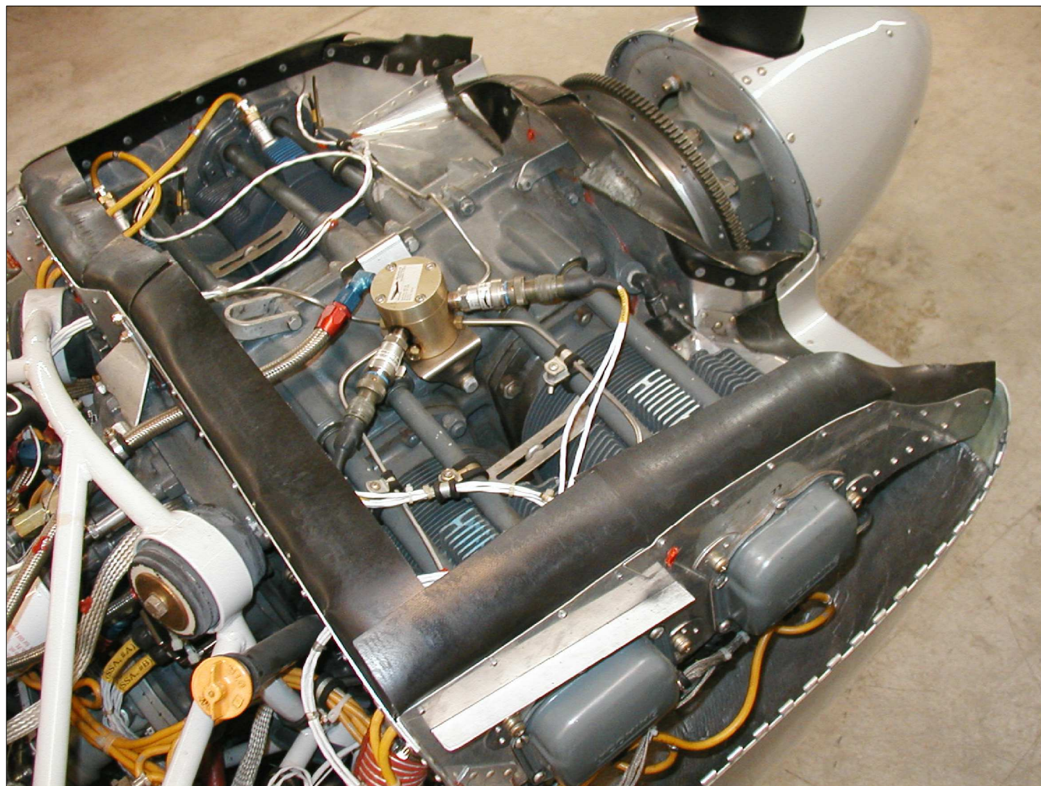
FIGURE 1: AIR SEAL FABRIC - RV-8 VIEW
