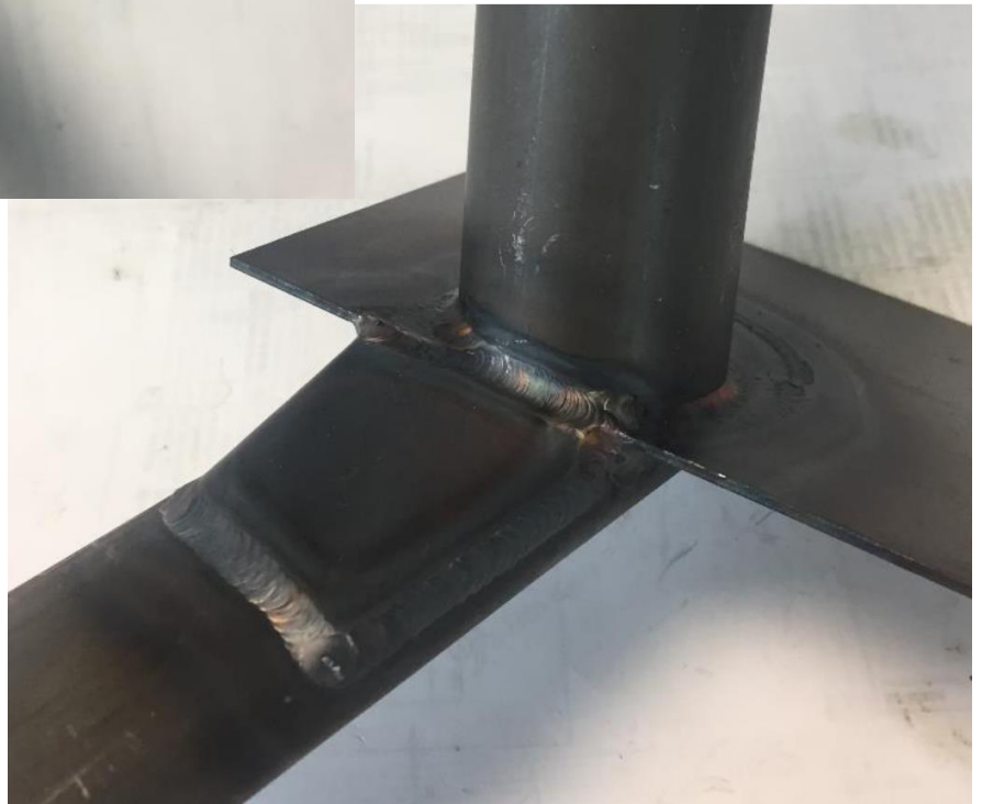
FIGURE 5: Welded assembly inboard
