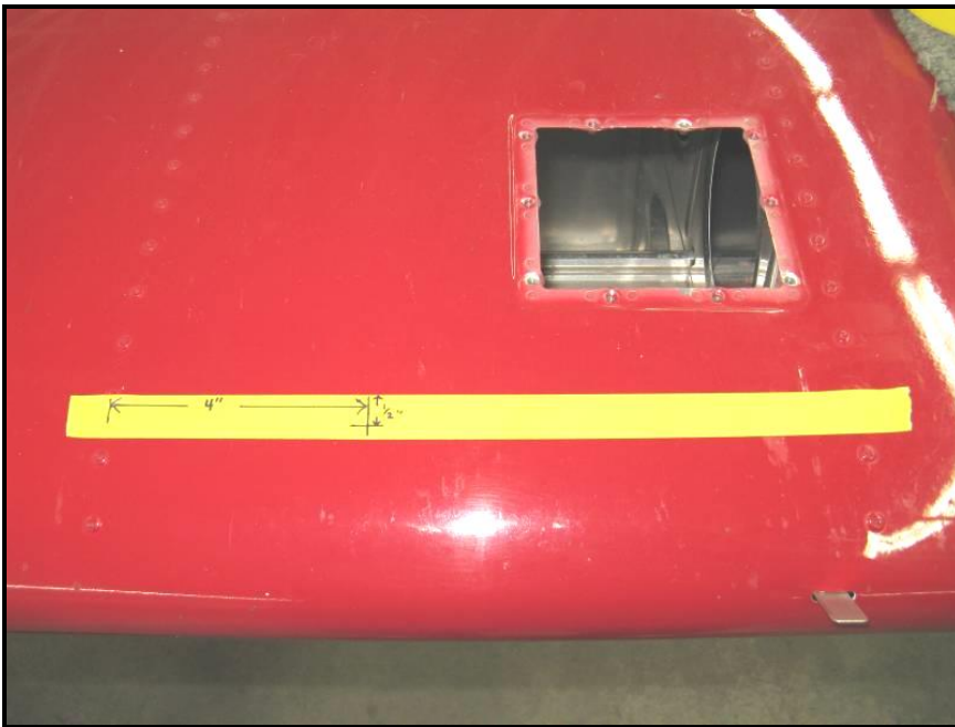
Figure 1: AOA Port location measurements on bottom of left wing. Note: Outboard end of wing is shown on the left.
