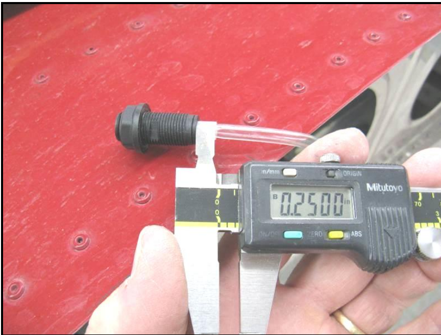
Figure 7: Plastic Adapter Tube fully inserted (1/2 in.) into the Wing FLF-00012, with the “fixed” nut shown on left. Not shown is the “non-fixed” nut already installed on the PT 1/8 CLR tubing and the tubing then inserted through the FLF-00012 mounting hole in the nose rib.
