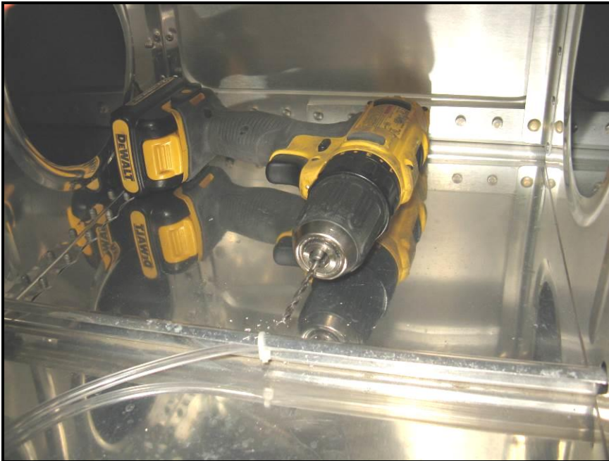
Figure 3: Drilling J-channel above the AOA port rivet for a tie-wrap.
