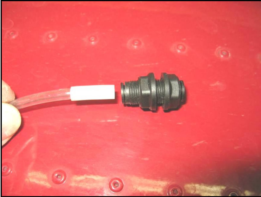
Figure 6: Plastic Adapter Tube made from PT-035X1/4, 3/4 in. long with “fixed” nut shown on right.
