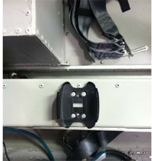
FIGURE 1: Spot mounting bracket installation
