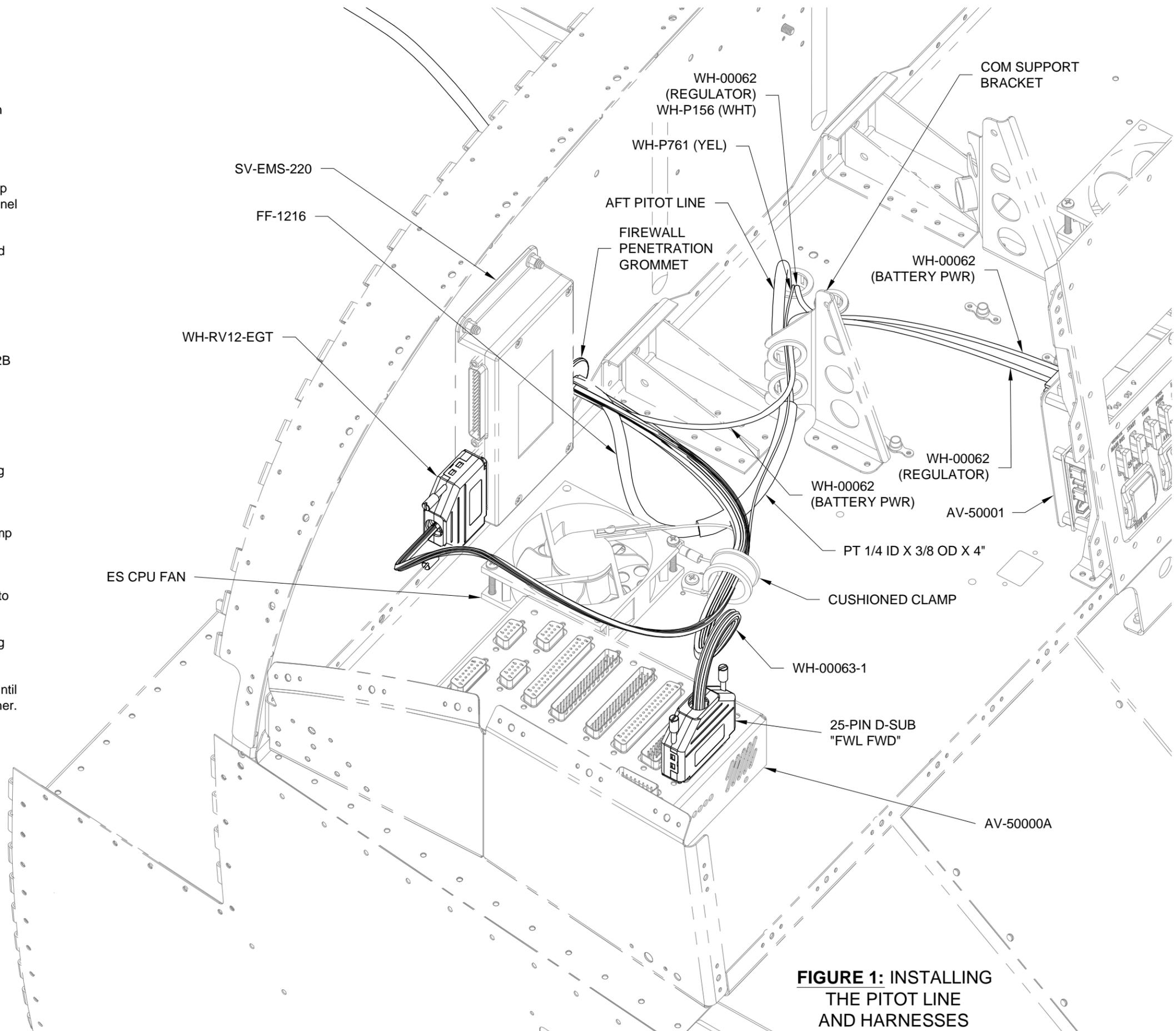
**FIGURE 1: INSTALLING THE PITOT LINE AND HARNESSSES**
