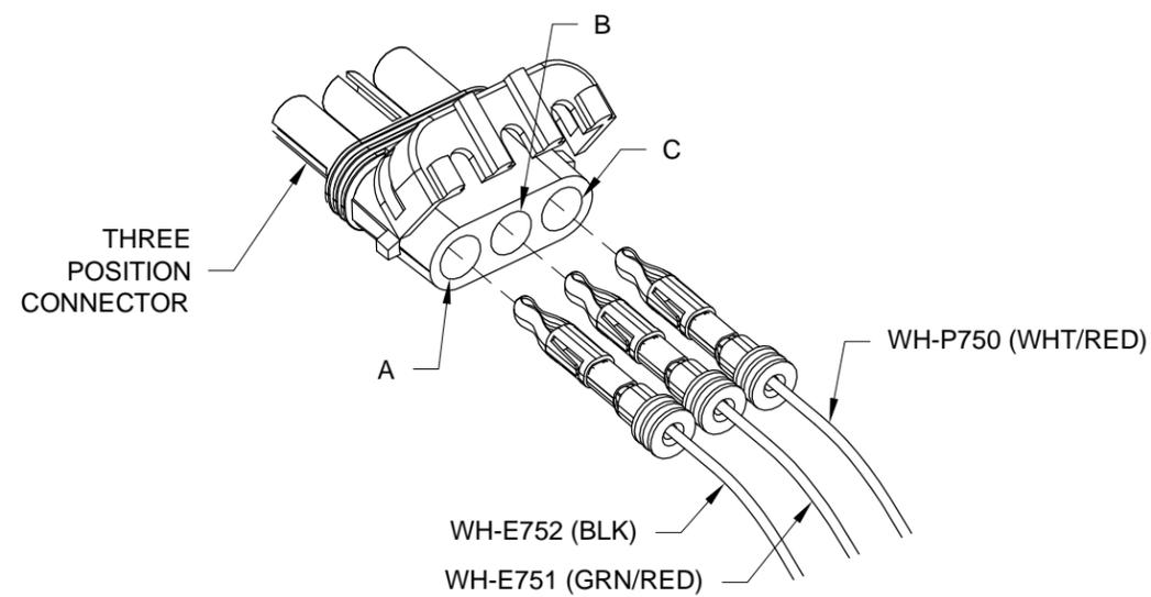
**FIGURE 1: INSTALLING WIRES IN THE CONNECTOR HOUSING**
