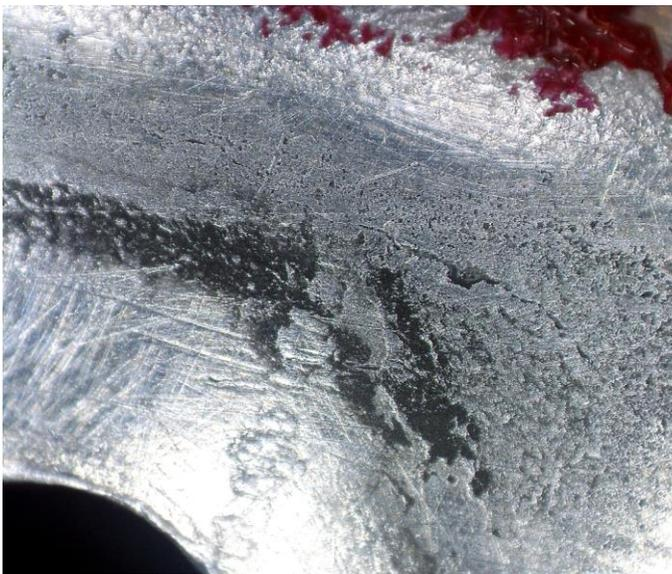
**FIGURE 2:** CRACK AFTER REMOVAL OF DYE PENETRANT
