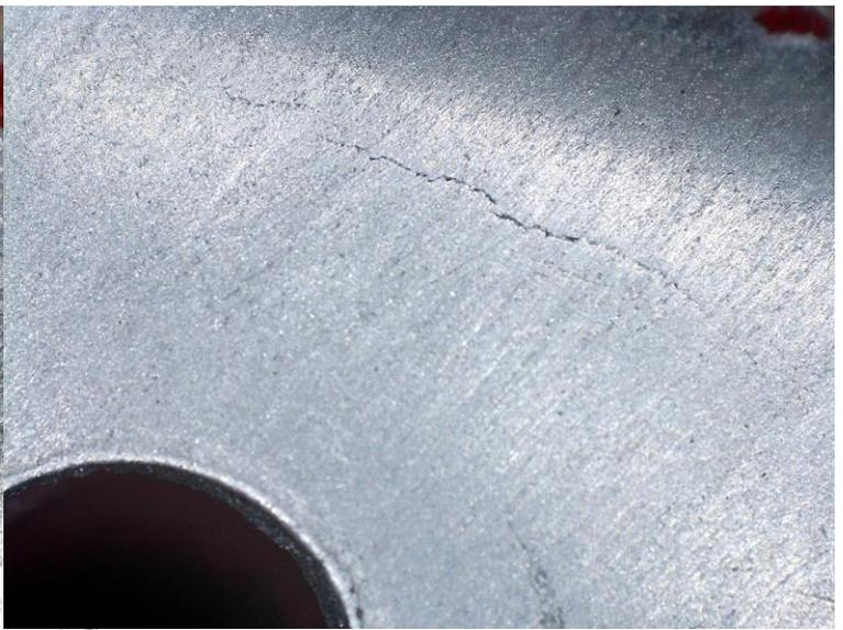
**FIGURE 3:** CRACK AFTER LIGHT SANDING WITH FINE GRIT PAPER
