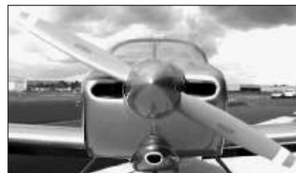
Because the metal prop is not as thick as the typical wood prop, a different spinner front plate is required.
