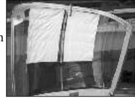
For the RV-14 canopy, the KOGER SHADE TU-WIDE is suggested. This may also be used in the 6/7/9 tip-up canopies if a wider shade is desired (adds about 2" each side to the standard tip-up shade).
