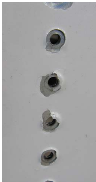
FIGURE 2: RIVET HEAD PAINT BUILDUP
