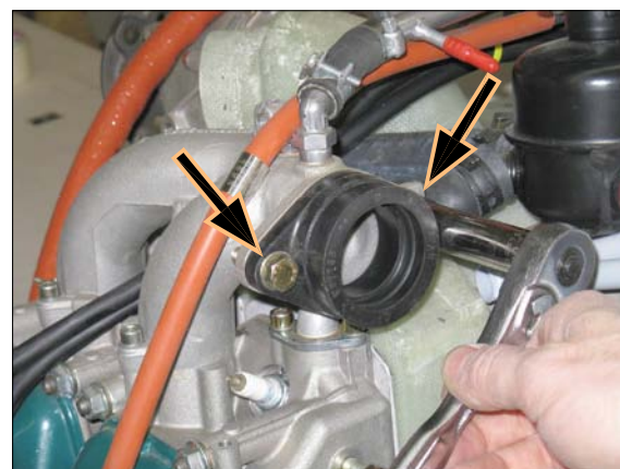
FIGURE 2: REMOVE CARBURETOR FLANGE ASSEMBLY
