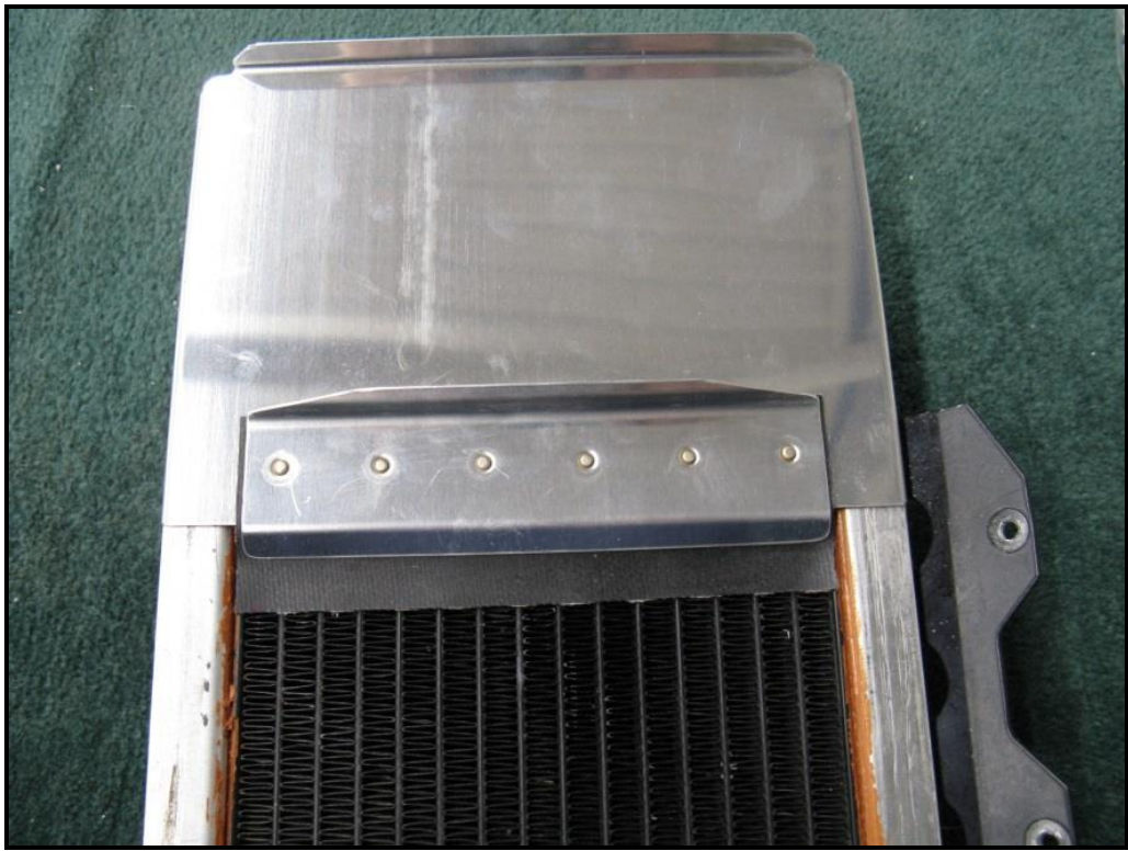
Figure 7: Seal trimmed to proper width.
