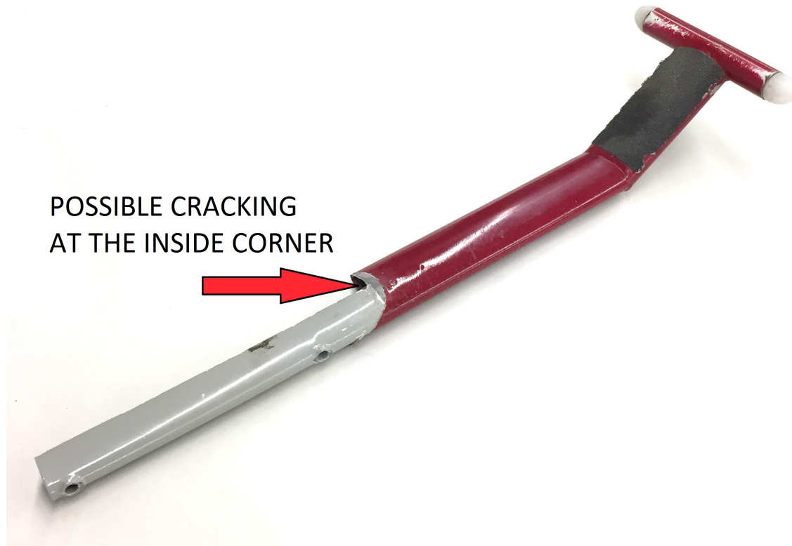
FIGURE 1: Location of possible cracking.
